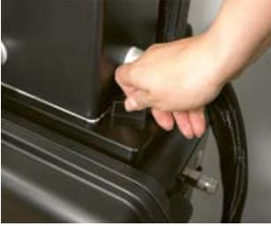
1. Place the measuring head to the holder at the top of the device. Remember to lock the measuring head in place with the locking knob.
