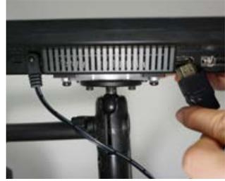
3. Connect the HDMI and the power cable to the display.
