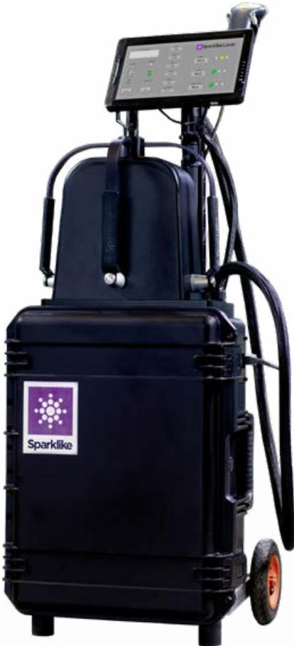
Thank you for choosing Sparklike Laser Portable 2.0™ to measure the gas concentrations on your insulating glass products. Sparklike Laser Portable™ is a unique product for non-destructive analysis, that measures even through coatings. Sparklike Laser Portable™ measures oxygen and the results can be converted to argon, krypton or additional insulating gas levels.
